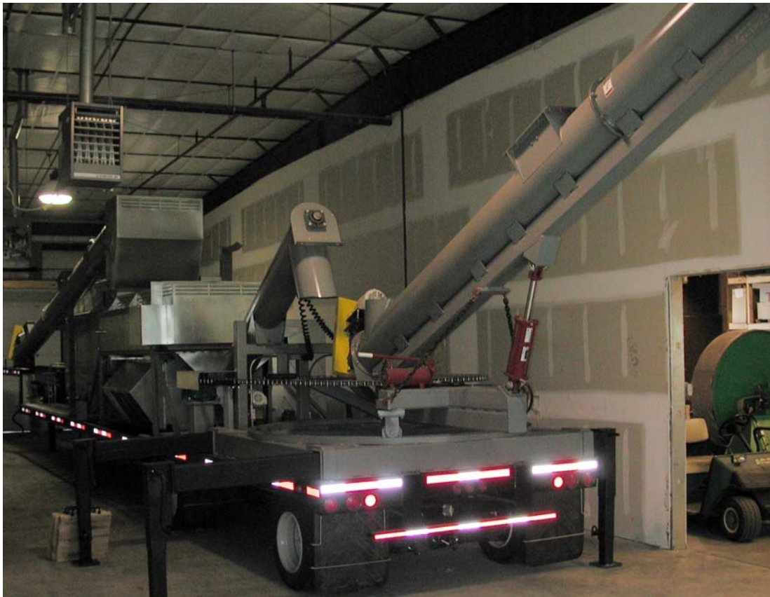
Figure 3. Decontamination and inoculation trailer end view. Rotating inoculation/pile-building conveyor raised in operating position.
