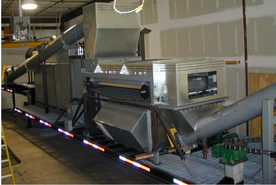
Figure 2. Chip cooling belt and blower system (partially assembled).
