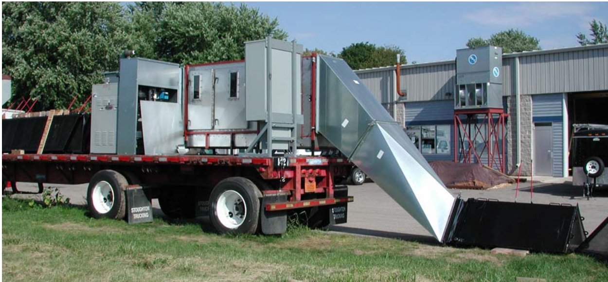
Figure 5. Ventilation/conditioning equipment trailer.
