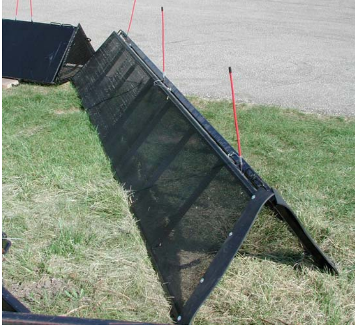
Figure 4. Section of portable under-pile ventilation tunnel.
