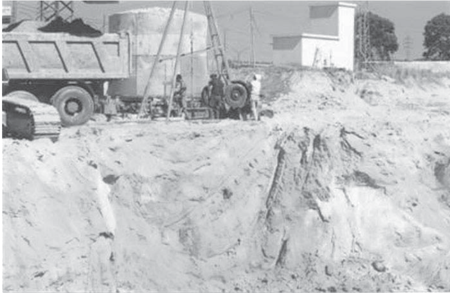
Figure 8.10 Overview of the weathered profile revealed in a fresh cutting on the experimental site
