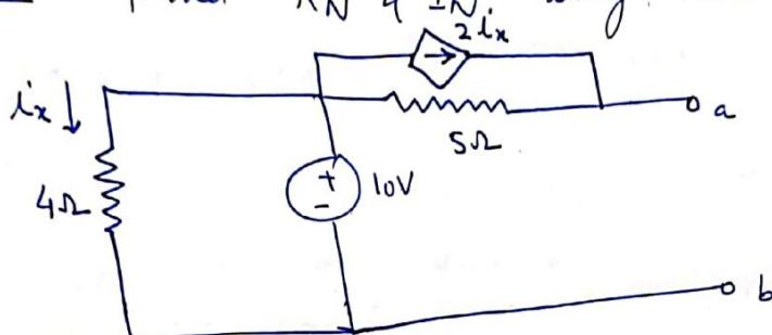
Sol. To find  $R_N$  we short ckt 10V source and let us apply a voltage  $V_0$  across as ( $= 1V$ ), the ckt as we get is,
