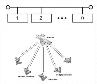
This system generally also allows possibility of addressing the packet to all destinations (all nodes on the network). When such a packet is transmitted and received by all the machines on the network. This mode of operation is known as *Broadcast Mode*. Some Broadcast systems also supports transmission to a sub-set of machines, something known as *Multicasting*.
