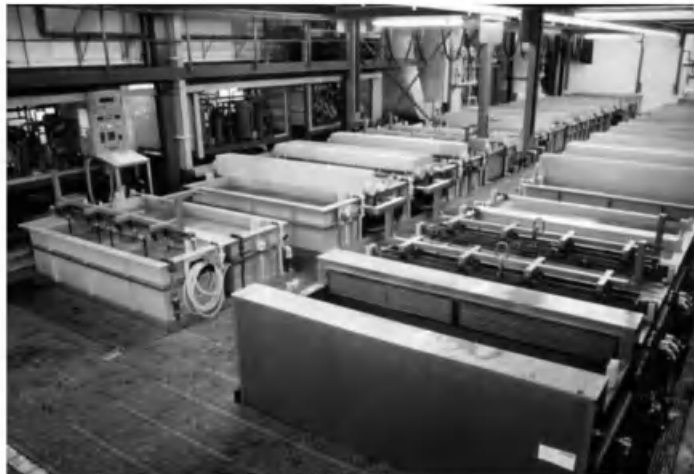
Figure 6.11 Bath sequence and anodic oxidation facility. Illustration courtesy of AHC Oberflächentechnik GmbH of the AIMT Group, Kerpen, Germany.
