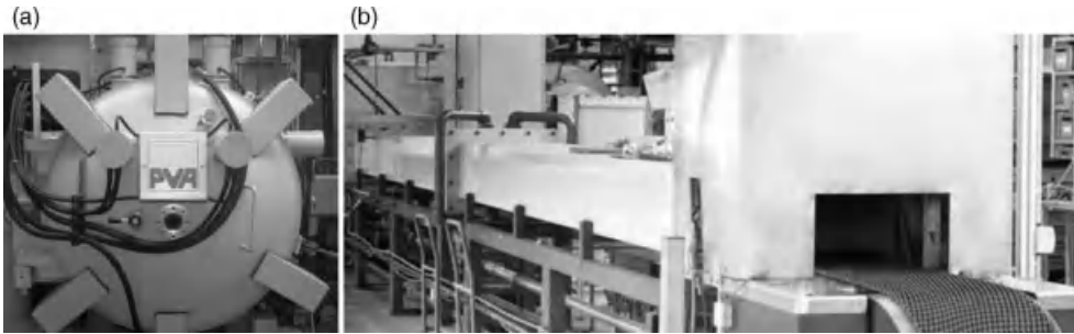
Figure 6.106 Furnace brazing systems. (a) High-vacuum brazing furnace; (b) Shroud gas brazing system. Illustrations courtesy of: (a) PVA TePla AG, Wettenberg; (b) Harnischmacher GmbH Fröndenberg.
