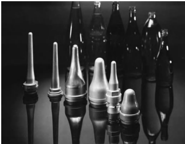
Figure 6.133 Borided extrusion dies (glass levels) for glass bottle production. Illustration courtesy of BorTec GmbH.
