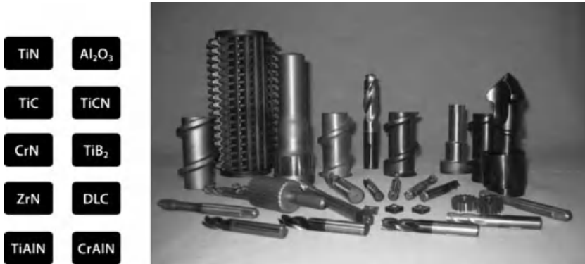
Figure 6.30 Commercial coating systems for tool coating and examples of their application. Illustration courtesy of IOT, RWTH Aachen.
