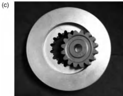
Si 3 N 4 equipped tool for precision forging (Source: IW, Leibniz Universität Hannover)
