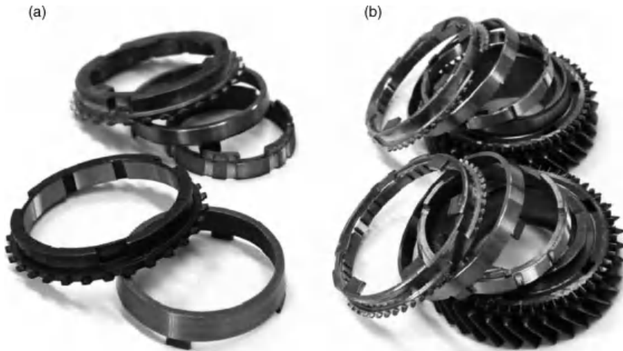
Figure 8.26 Synchronizer systems currently in use. (a) Single- and double-cone synchronizers; (b) Triple-cone synchronizers.
