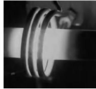
Figure 6.107 Induction brazing for the internal coating of cylindrical parts.
