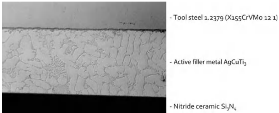
Figure 6.115 Active-brazed ceramic-steel compound, brazed at 1000 °C for 10 min in vacuum. Illustration courtesy of IOT, RWTH Aachen.)
