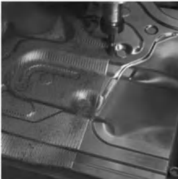
Laser deposition welding. Tool and mold making. (Source: Fraunhofer IPT, Aachen)
