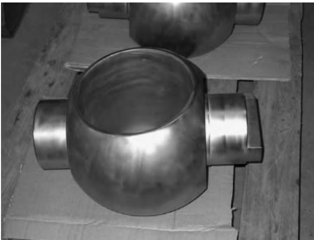
Figure 6.134 Chromized ball valve with a diameter of about 80\ \text{cm} . Illustration courtesy of Chromin, NL.
