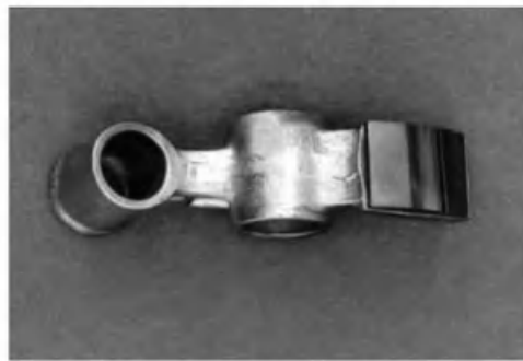
Si 3 N 4 equipped rocker arm of a Diesel engine (Source: IOT RWTH Aachen)
