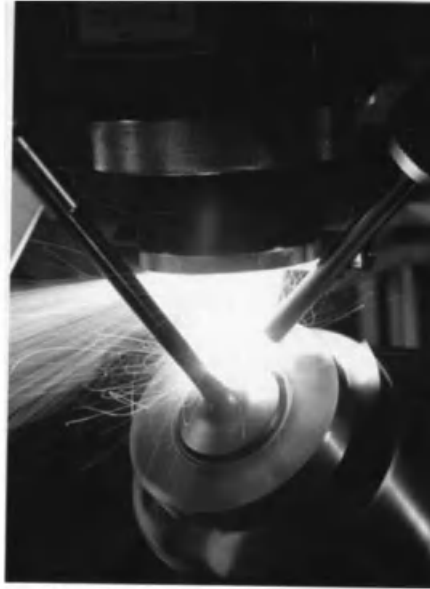
Laser deposition welding. Stellite coating of a valve seat (Source: Fraunhofer IWS, Dresden)
